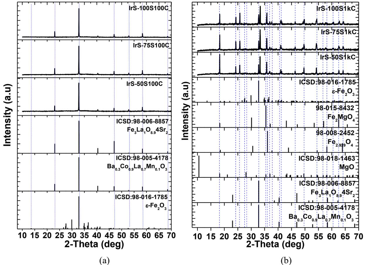
**Figure 2.** XRD pattern of iron sand with variation volume of HCl of 50 ml, 75 ml and 100 ml sintering at 100 °C (a) and 1000 °C (b).
