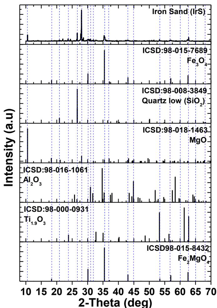
**Figure 1.** XRD pattern of Iron sand (Irs) after mechanical decantation.
